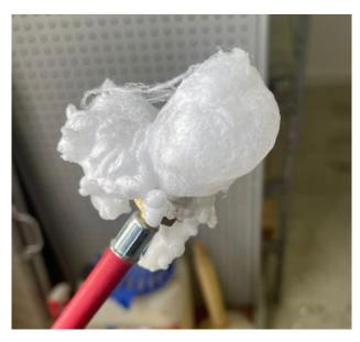
Although the reasons have not been made 100% clear, this phenomenon can occur due to humidity and high temperatures, for example when gas bottles are exposed to direct sunlight or there is a leaking pressure valve.
